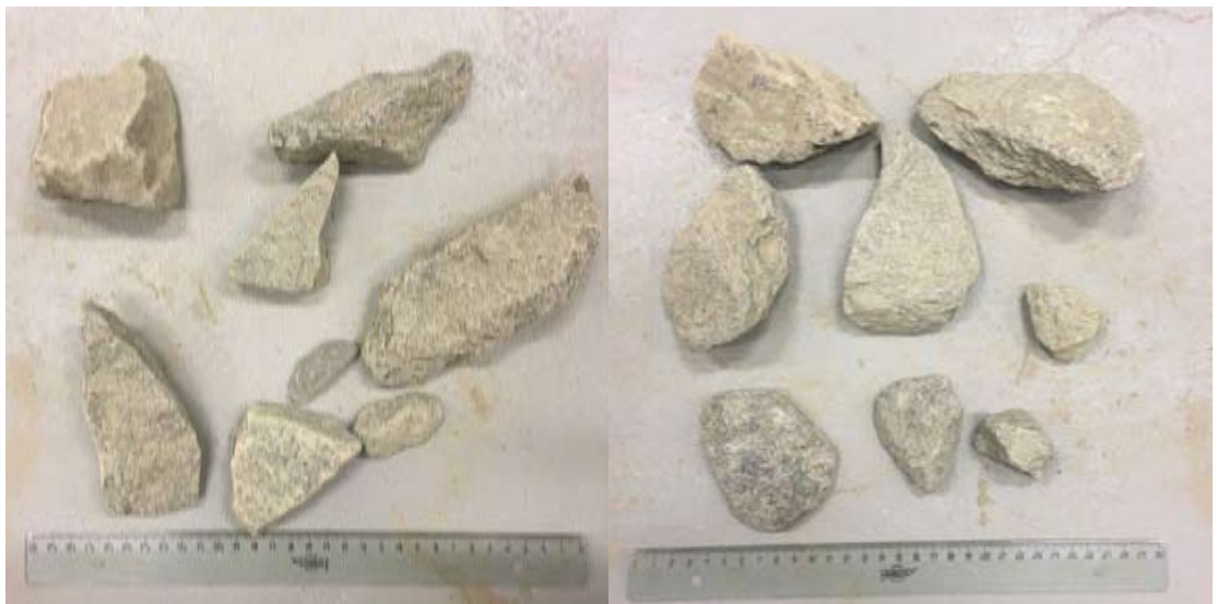
Figure 7 Rounding of the rock particle after repeated testing. Left: before tests; Right: after four tests. (Note: the rocks are not the same before and after four tests).
