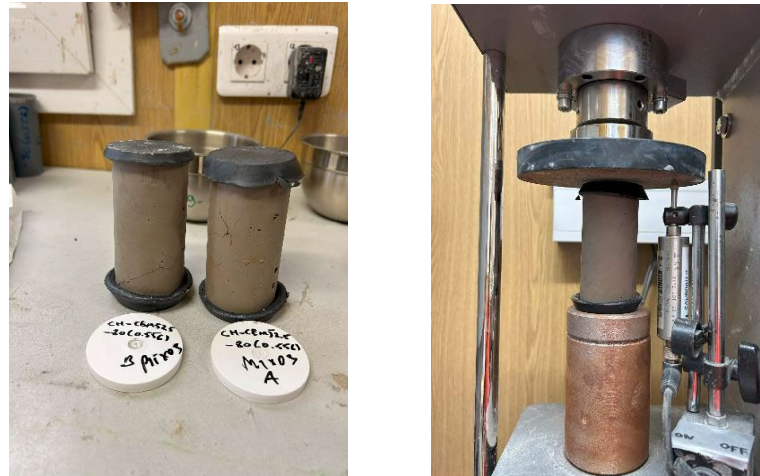
Figure 6 UCS test on specimens with strain-controlled loading device and failure of specimens
