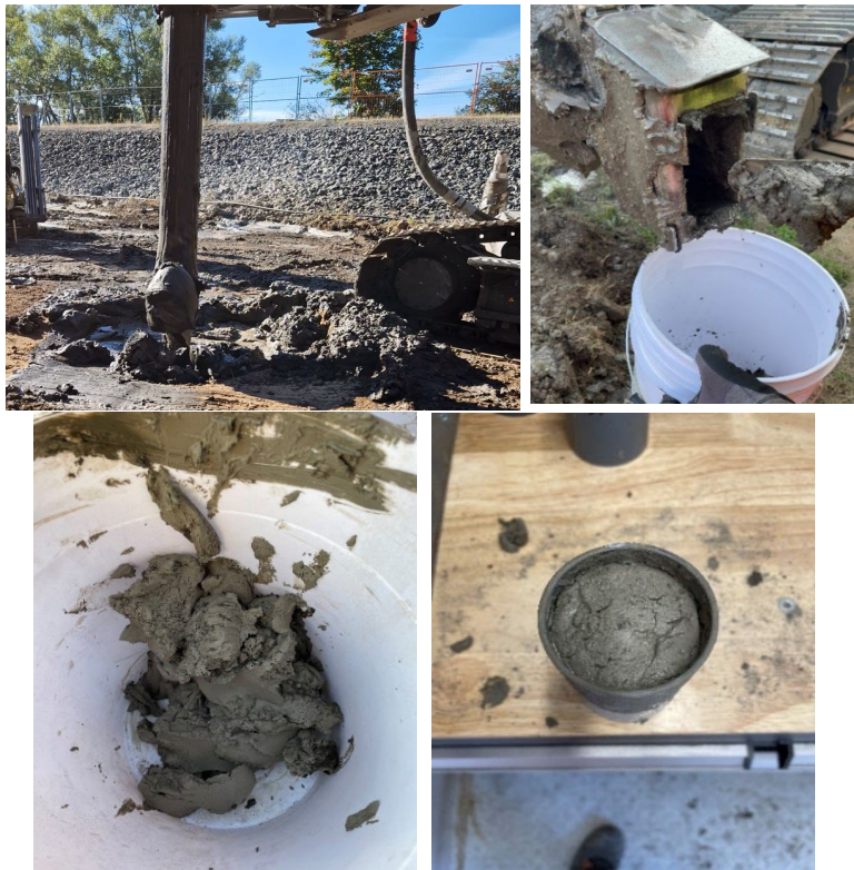
Figure 11 Wet grab sampling with a tool attached to the rig and specimen preparation
